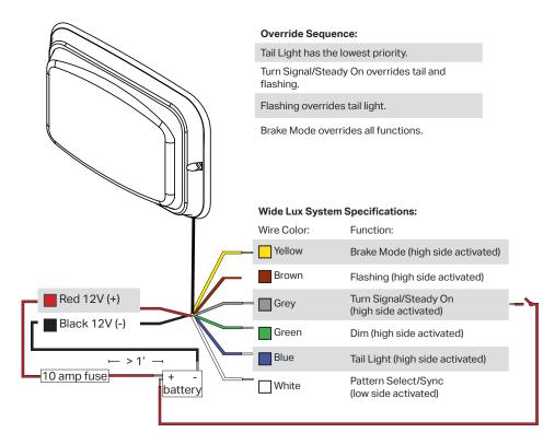
Step 1: In order to activate the unit, extend the red, 12V+ wire to the 12V+ post of the vehicle's battery. Extend the black, 12V-wire to the ground post of the vehicle's battery.
