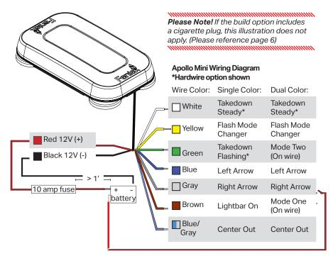
Step 1: In order to activate the unit, extend the red wire to the 12V(+) post of the vehicle's battery. Extend the black wire to the ground post of the vehicle.
