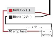
**Warning!** All user supplied wires connecting to 12V (+) or 12V (-) must be sized to supply 100% of the maximum current and properly fused at the power source with the correctly rated fuse. Avoid routing wires in the deployment area of the vehicle air bag or any other potentially hazardous locations.
