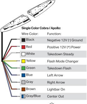
Step 1: To activate the unit, extend the red, 12V (+) wire to the 12V (-) post of the vehicle's battery. Extend the black, 12V (-) wire to the ground post of the vehicle's battery or chasis.
