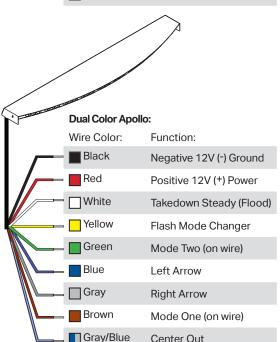
Important! Do not wire this unit to an alternative power supply, such as a AC to DC converters. Wire only as instructed. The red, 12V (+) wire should only to the vehicle's battery or to a 12V (+) switch post. Failure to do so may damage the unit and void warranty.
